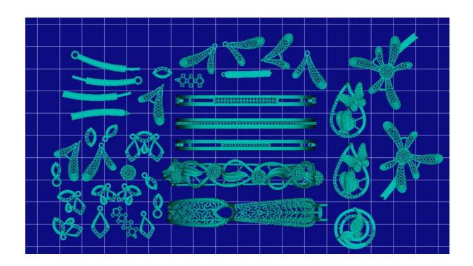
In-house developed software for 1-click auto- placement and 1-click slicing for DLP 3D Printers.
