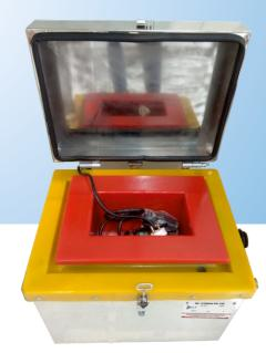
Doit Industries Rectangular vibrators are devices designed to perform smoothing, finishing, polishing of Jewellery of Variable range of sizes using Abrasive Materials with vibration effect of the Vibrator. The Motion of the Abrasive Material along with the Action of Water and detergent results in top grade finishing.
