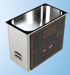
Ultrasonic machine is an indispensable system for jewellery. Cleaning, as manufacturing progresses, becomes more critical. As cleaning is to be done in intricate areas, under stones, Doit Industries research and development has created ultrasonic machine with effective cavitations which causes formation of minute bubbles in cleaning liquid and thus cleaning dirt from minutest places. You can also achieve very effective cleaning with more than 90% power saving and faster cleaning
