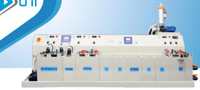
Doit Industries galvanic plant built entirely of polypropylene for working tanks of 30 or 40 litters as per Requirement, it's suitable for rhodium, degreasing, gold Micron or Flash Bath with washing and recovery tanks.
